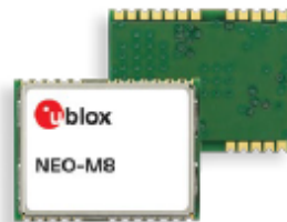
Figure 4 NEO-M8Q-0 GPS Module
