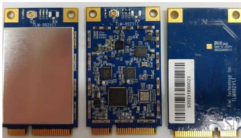
Figure 2 KIWI TLM992 8CH LoRa Module
