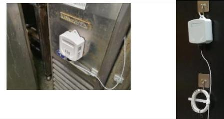
2.7 Place the sensor at temperature-monitoring position as you need or refer to Kiwi's suggestion on chapter-9) Sensor position suggestion.
